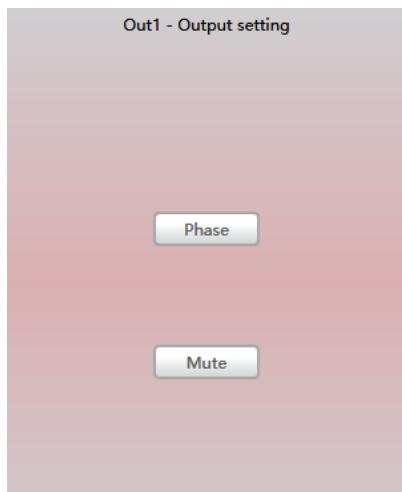
**Phase:** The phase of the audio signal is reversed by 180°.
