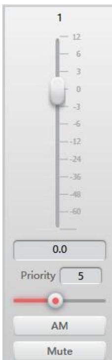
**AM:** Each Channel has an auto mix on/Off button that needs to be turned on for Channel participating in auto mix. It can also be turned off, and the Channel does not participate in automatic mixing.
