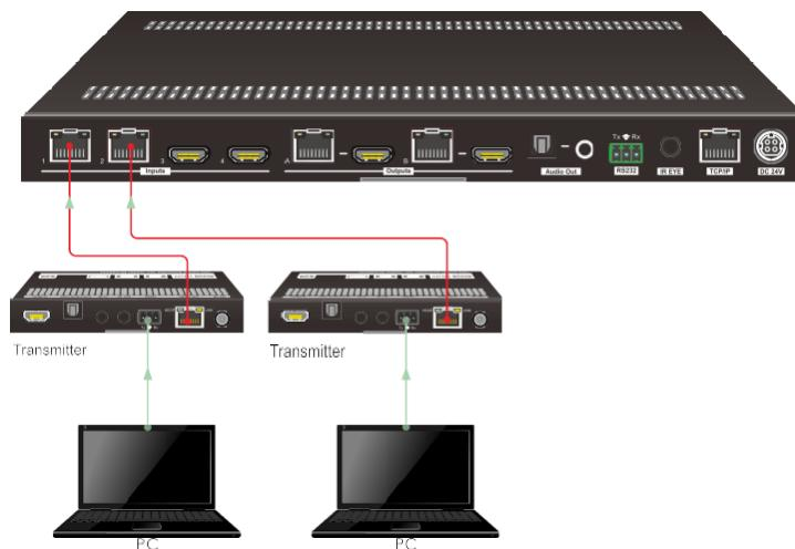
3) To control the matrix switcher from remote receiver location, please connect one or two PCs to the RS232 ports of HDBaseT receivers with the 3-pin to DB9 RS232 cables. The matrix switcher can be controlled by any one of PCs, the connection diagram is shown as below:
