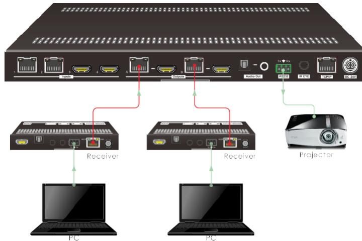
2) To control remote third-party device from local matrix switcher location, first determine which HDBaseT receiver is connected to. Next, connect a PC to the RS232 port of matrix switcher, then connect a third-party device (e.g. projector) to the RS232 port of HDBaseT receiver, the connection diagram is shown as below:
