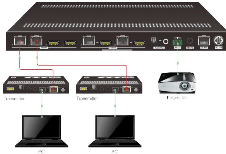
2) To control remote third-party device from matrix switcher location, first determine which HDBaseT transmitter is connected to. Next, connect a third-party device (e.g. projector) to the RS232 port of HDBaseT transmitter, then connect a PC to the RS232 port of matrix switcher, the connection diagram is shown as below:
