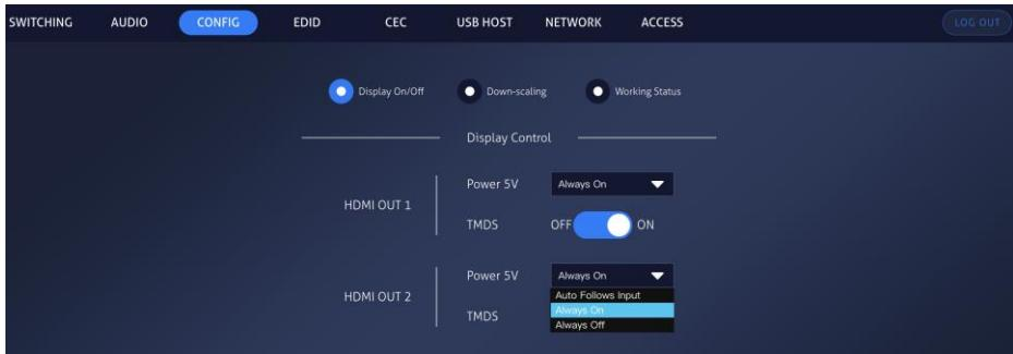
HDMI output with controller. Can turn ON and OFF 5V+ (HPD) when no sources are showing image. Same goes with TMDS+ Clock signal.
