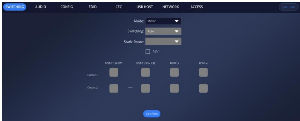
The latest source connected will be routed to both outputs.
