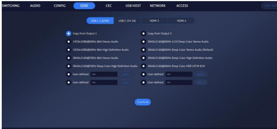
Copy the EDID from Output1 or Output2 or select built-in 8 EDID for the selected input source.
