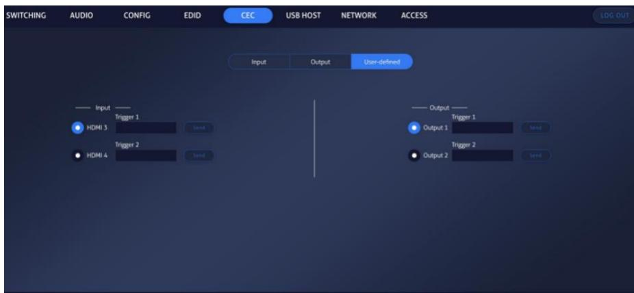
The switcher also provides user-defined CEC functions, the CEC command can be edited and saved in the Trigger box.
