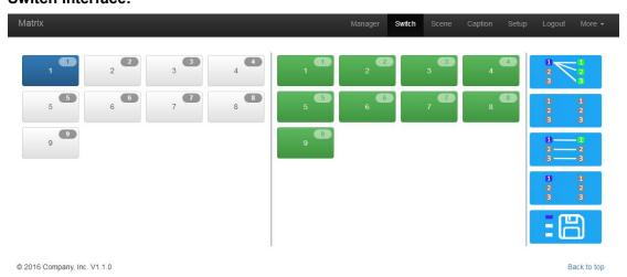
The left side of the long string is input area: Mini99 will have 9 buttons, Mini1818 has 18 buttons, Mini3636 will have 36 buttons. The right side is output area, the buttons are the
