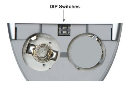
It is important that the IR channel selected on the remote, match the IR channel on the GefenTV 4x1 Switcher for HDMI 1.3 for proper operation. For example, if you set both DIP switches on the remote to the down position (toward the "1" and "2"), IR channel 0, you must set the GefenTV 4x1 Switcher for HDMI 1.3 to use IR channel 0.
