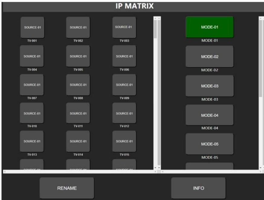
**Receiver devices** panel on left, configure receiver's device name, video source device. The display device button aligned in the sequence of IP address.
