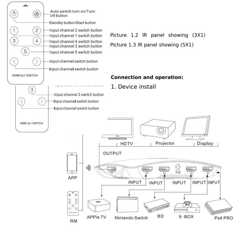
1. To use HDMI cable to connect the HD source with the HDMI input port of device.
