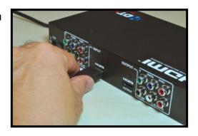
b) YPbPr – Connect the YPbPr cables, matching the colors between the connectors and adapters (top row - shown right). There are two audio connectors for the L-R audio connectors below the YPbPr adapters. Attach the other ends of all the cables to your HDTV.
