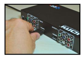
b) **YPbPr**— YPbPr cables have 3 connectors, each color coded (green, blue and red). Simply match the colors on the connectors with the color coded adapters on the HDTV Recorder (top row - shown right).
