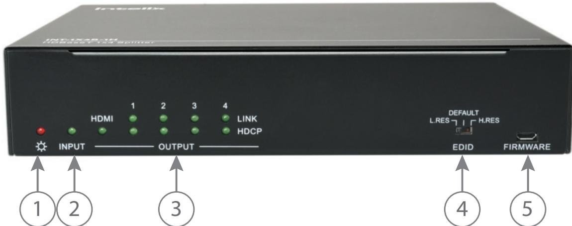
1. **POWER LED** - Illuminates solid RED when power is properly applied
