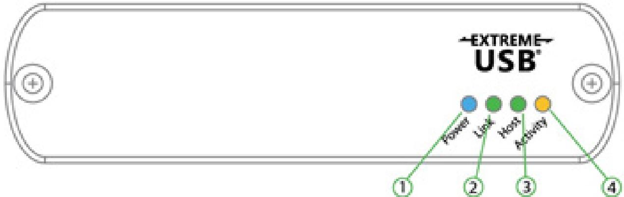
1. Power LED (Blue) :When the blue power LED is on the IPEX-USB2-H has power. When the LED is off no power is supplied by the host computer.
