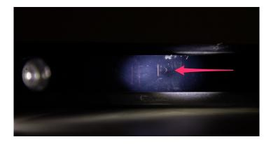
3. Using the included sticky tape attach the IR to the source device
