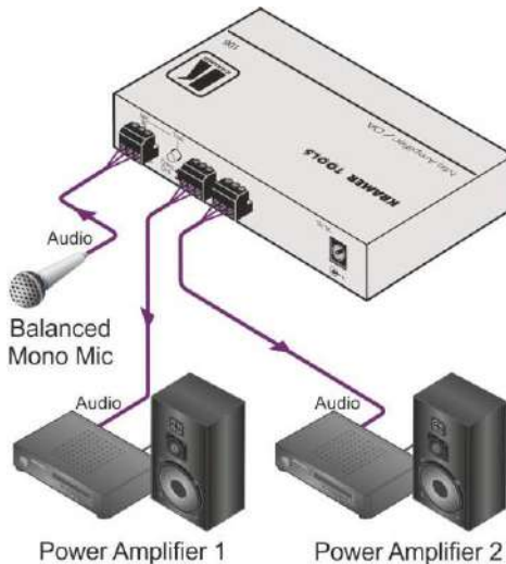
Figure 2: Connecting the 106 Mic Amplifier/DA
