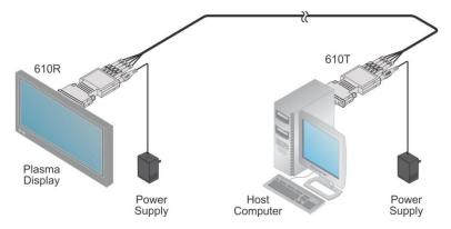
Figure 4: Connecting the 610T/610R Detachable Optical DVI Transmitter/Receiver
