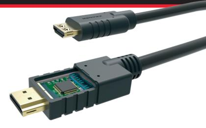
The Kramer CA-HM active HDMI™ copper cable provides a perfect cable solution for delivering HDMI signal over long distances. CA-HM runs 18Gbps up to 20m (66ft), 10.2Gbps up to 25m (82ft), and 6.75Gbps up to 30m (98ft). The innovative technology utilized in the cable's connector features superior equalizing and signal compensation to meet the most demanding challenges in Pro AV installations.
