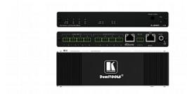
FC-404NETxl is a hybrid, analog and Dante, audio cross-connect mixer. Input audio, either analog lines/microphones or Dante audio over IP channels, are mixed and cross-connected to the analog audio output lines and/or Dante audio over IP output streams. The mixer accepts PoE via its network connection
