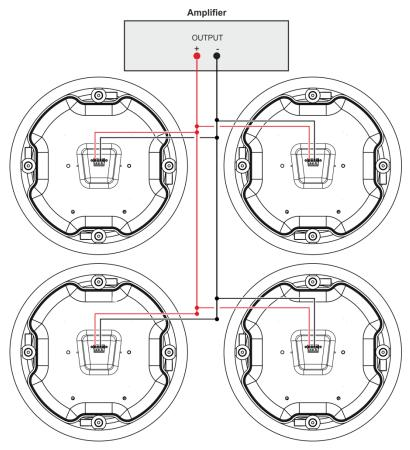
Figure 10: Square Layout Parallel Wiring
