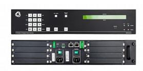
MTX3-16-M is an intelligent and high performance 16x16 modular matrix for switching and distribution of multi-format audio-visual signals. The chassis includes a CTRL central control card with secured LAN connectivity for remote management and control, and has eight card slots for flexible insertion of modular matrix cards, accommodating matrix cards with quad or dual ports of either input or output multi-format signals
