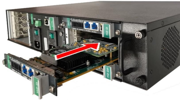
Figure 7: Input / Output Card Installation on the MTX3-16-M
