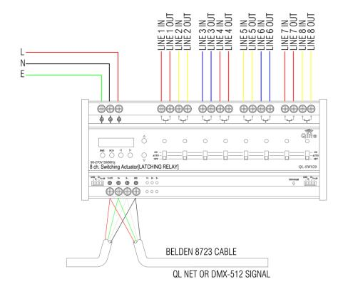
Fig 2. Module Connections
