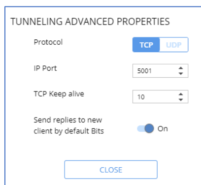
Figure 29: Setting Tunneling Advanced Properties
