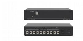
The VA-102P5 is a 10-output power supply that powers 5V DC powered devices. The VA-102P5 can supply a maximum of 1.8A of current to each of ten devices for a total of 18A. The power supply is especially useful in high-population installations for saving space and eliminating a large number of 5V DC power adapters. The MD model is suitable for medical applications
