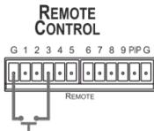
To select input 3, momentarily connect the 3 PIN to the G PIN.
