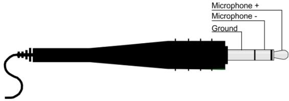
Figure 6: Microphone Pinout
