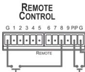
To select PIP input 8, connect the PIP PIN to the G PIN and, within 3 seconds, momentarily connect the 8 PIN to the other G PIN.
