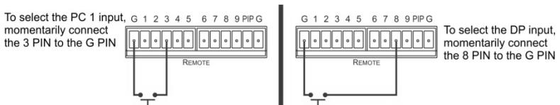
Figure 36: Connecting the Contact Closure Remote Control PINs
