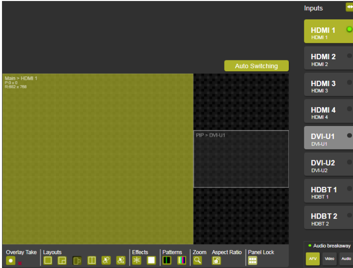
Figure 40: Routing and Scaling Page – Before Swapping Pictures
