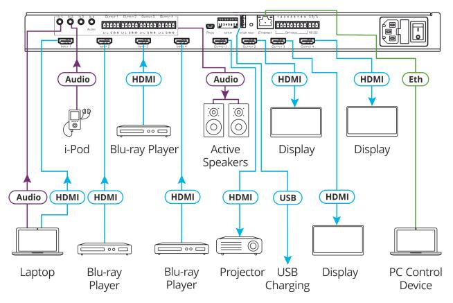
Figure 3: Connecting to the VS-44UHDA Rear Panel
