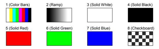
Figure 10: VS-44UHDA Embedded Patterns
