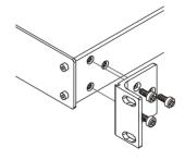
2. Place the ears of the **VS-44UHDA** against the rack rails and insert the appropriate screws (not provided) through each of the four holes in the rack ears.
