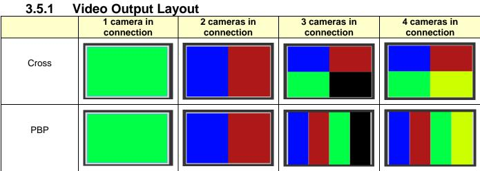
If there are three connected cameras, they will be displayed in a 4-grid layout, with one grid showing a black screen.
