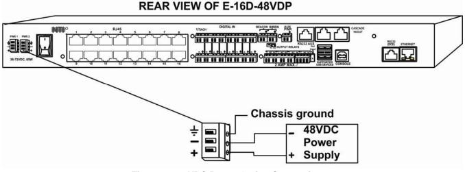
Figure 20- 48VDC Power Option Connections
