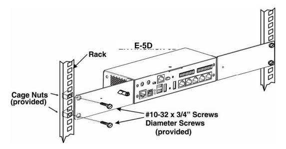
Figure 4- Mount E-5D/2D in a rack
