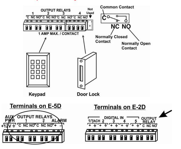
Figure 13- Install additional devices to output terminals
