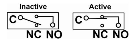
Figure 54- Output Relay Contact State
