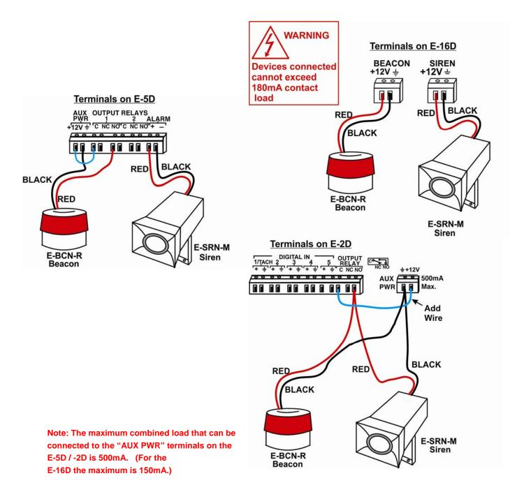
Figure 12- Connect visual and audible external indicators
