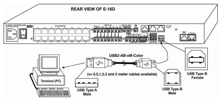
Figure 15- Connect a terminal using USB Console port
