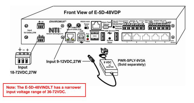
Figure 22- Power connections on E-5D-48VDP
