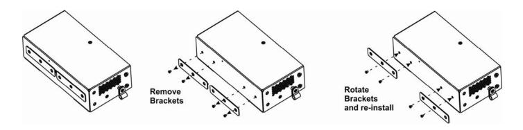
Figure 3- Rotate the tabs for Zero-RU mounting
