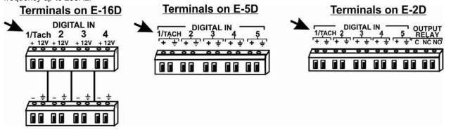
Figure 51- Connection that supports Tachometer Sensor
