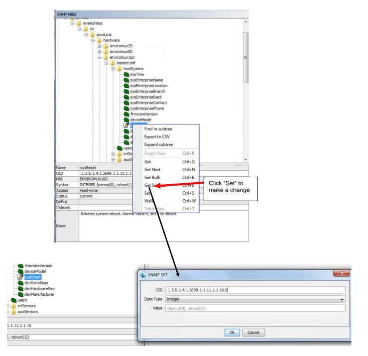
Figure 148- Use SNMP to reboot the ENVIROMUX
