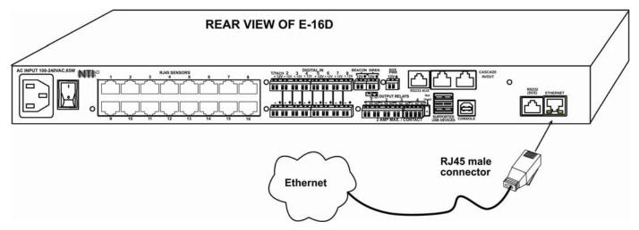
Figure 16- Connect ENVIROMUX to the Ethernet
