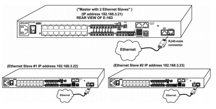
Figure 99- Cascade configuration with Ethernet slaves
