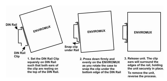
Figure 6- DIN Rail Mount with metal clip
