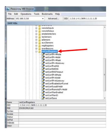
Figure 149- Network Configuration topics through SNMP
