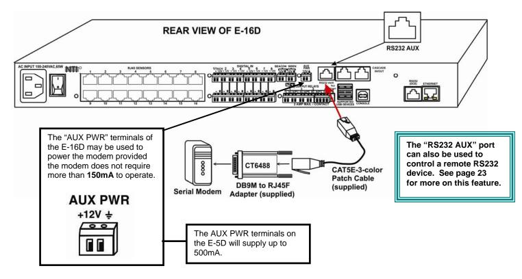
Up to 1000 feet of CAT5E (350Mhz) cable may be used at a baud rate of 115,200bps.
