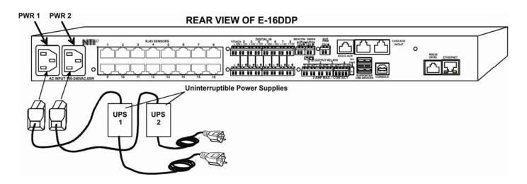
Figure 19- Power connections for ENVIROMUX with Dual Power Option
