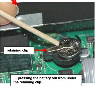
6. Re-install the new battery by reversing the process. (**CR1225** for E-2D/5D, **CR2032** for E-16D) With the E-2D/5D, be very careful not to lift up to hard on the retaining clip. Lift only far enough to slip the edge of the new battery under it and slide the battery back into place.
