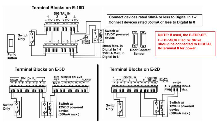
**Figure 9- DIGITAL IN Terminal Connections**
