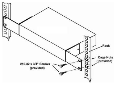
Figure 2- Mount ENVIROMUX in a rack
