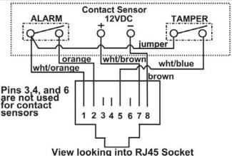
Figure 8- Contact sensor wired to RJ45 socket
