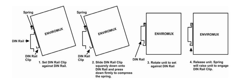
Figure 5- Mount E-5D/2D to DIN rail- plastic clip
