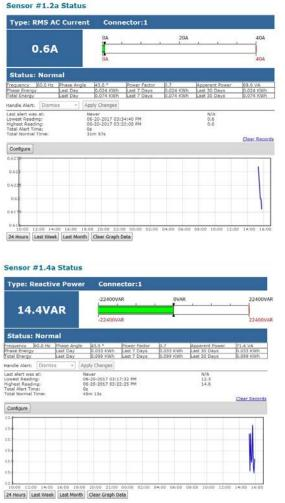
Click on the "Configure" button on any Status Page to display the Configuration page for any sensor.
