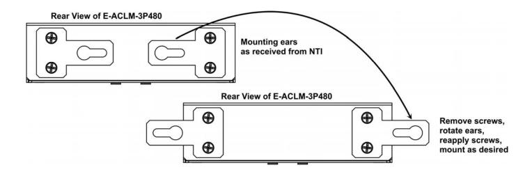
To mount multiple E-ACLM-3P480 in close proximity to the E-16D, install an extension rail kit (NTI E-RL-16D - sold separately) and mount E-ACLM-3P480 as seen in the illustration below.
