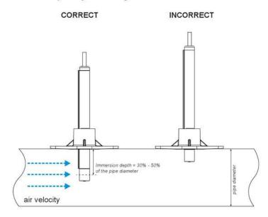
If the sensor probe is installed without a mounting flange, make sure the air velocity sensor is aligned parallel with the air stream.
