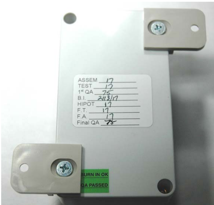
Brackets and screws installed.
