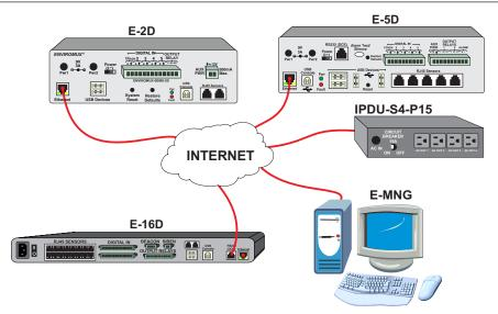
How to connect and control up to 3,000 E-2D/5D/16D, E-SEMS-16(U), and IPDU-S4/8 units via Ethernet
