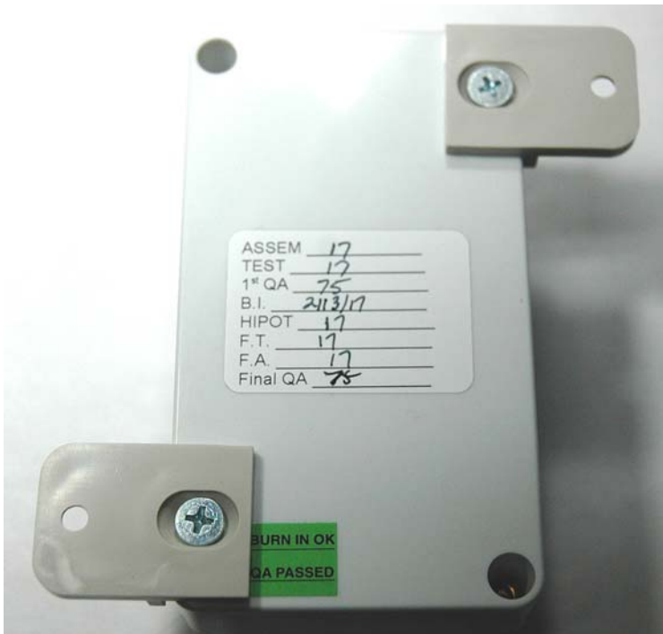
Brackets and screws installed.
