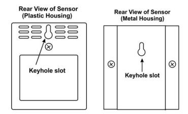
Figure 1- Keyhole slot for standard mounting
