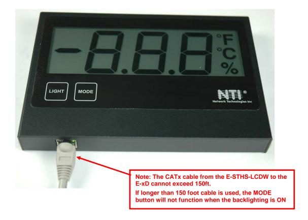
The cable from the ENVIROMUX will attach to the sensor at the RJ45 port on the bottom of the E-STHS-LCDW. The E-STHS-LCDW will be powered by the ENVIROMUX Monitoring System through the CATx cable. We recommend using CAT5/5e/6/6a cable (minimum 24 AWG) up to 150 ft (45.7 m) long.
