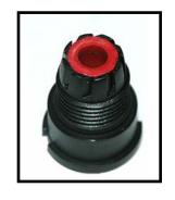
2. Strip the CATx shielded cable jacket (6mm-7mm O.D.) approximately  $\frac{1}{2}$ " and insert the cable through the sealing nut, screw nut, and housing. (Note: Heat shrink tubing can be applied to cable to increase the O.D. of the CATx cable to 6mm-7mm.)
