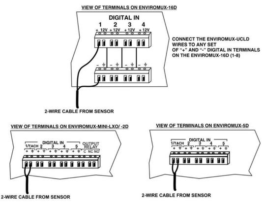
CONNECT THE ENVIROMUX-UCLD WIRES TO ANY SET OF "+" AND "  $\stackrel{\leftarrow}{\div}$ " DIGITAL IN TERMINALS ON THE ENVIROMUX-MINI-LXO, ENVIROMUX-2D OR ENVIROMUX-5D
