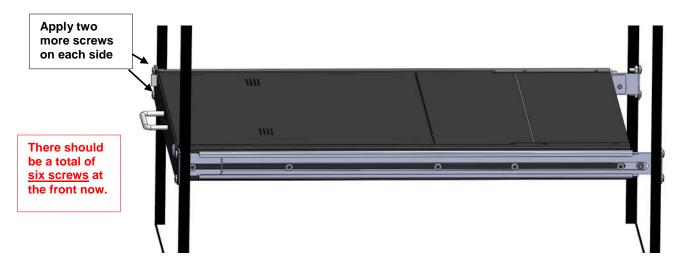
Figure 7- Secure the RACKMUX
