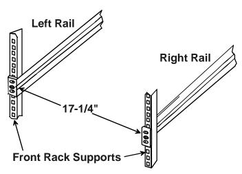
Figure 5- Adjust distance between rails
