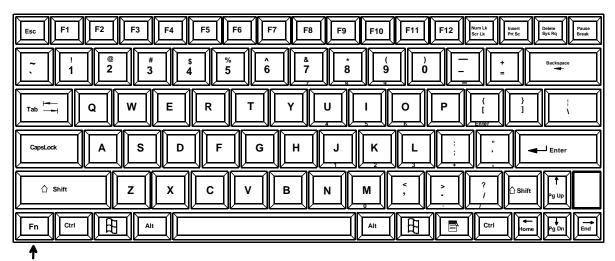
Function Key to enable additional key functions
