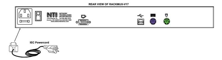
Figure 14- Connect the power cord
