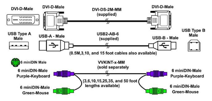
Figure 12- Cables used for RACKMUX with DVI video support
