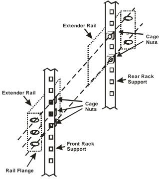
Figure 3- Install cage nuts
