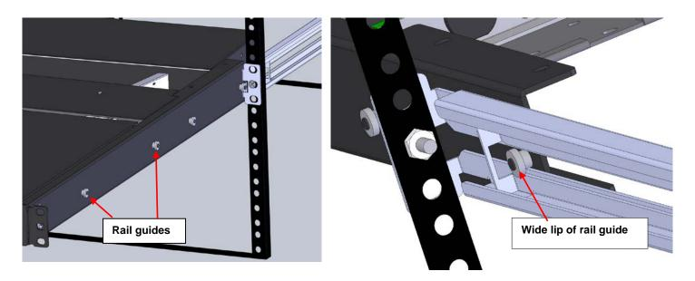
Figure 6- Slide the RACKMUX into the rails
