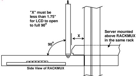
Figure 8- Position RACKMUX with clearance to open
