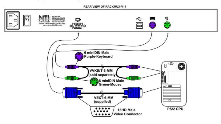
Figure 10- Connect a PS/2 CPU
