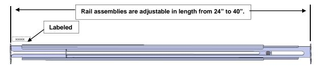
Figure 2- Adjustable rail depth
