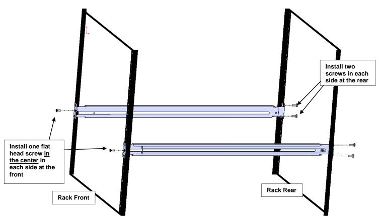
Figure 4- Install rail assemblies
