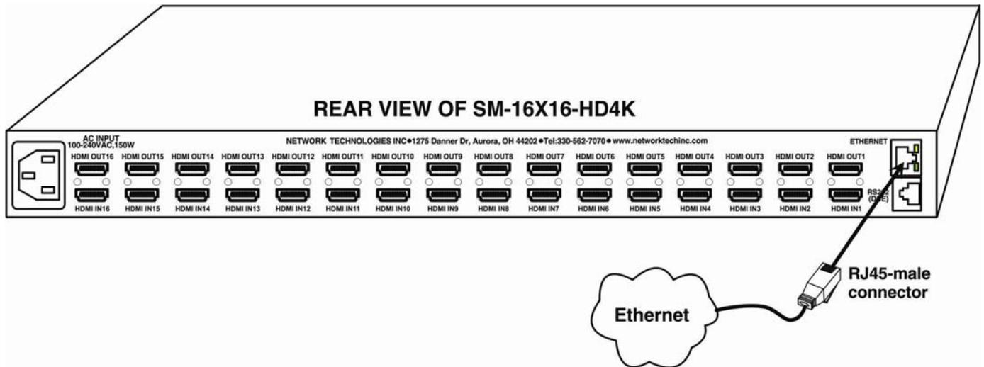
Figure 5- Connect VEEMUX to local area network
