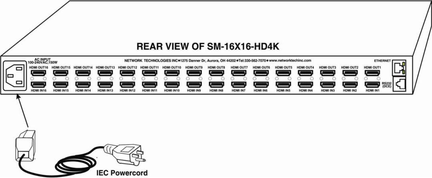
Figure 6- Attach AC power cord to VEEMUX
