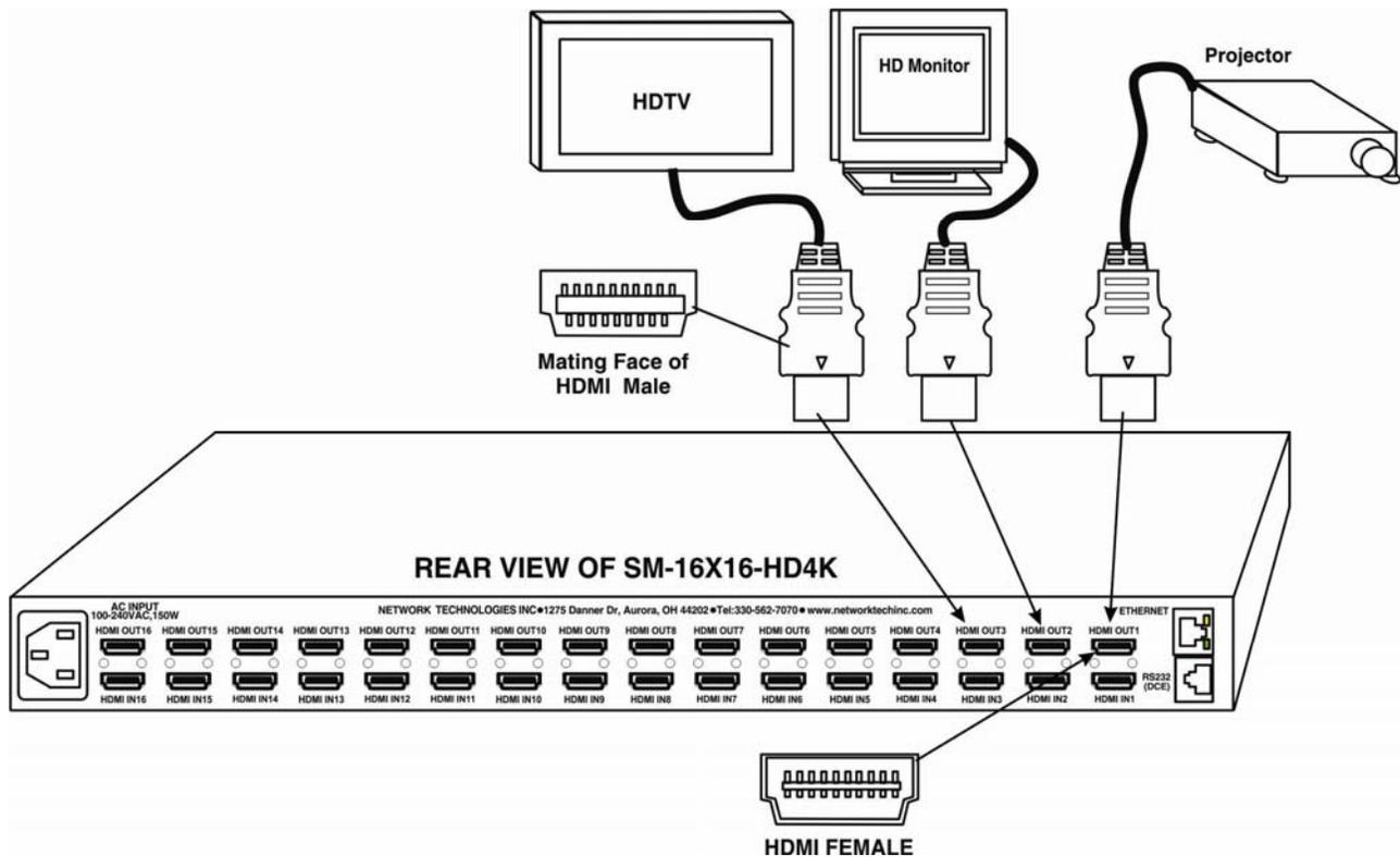
Figure 3- Connect display devices to VEEMUX
