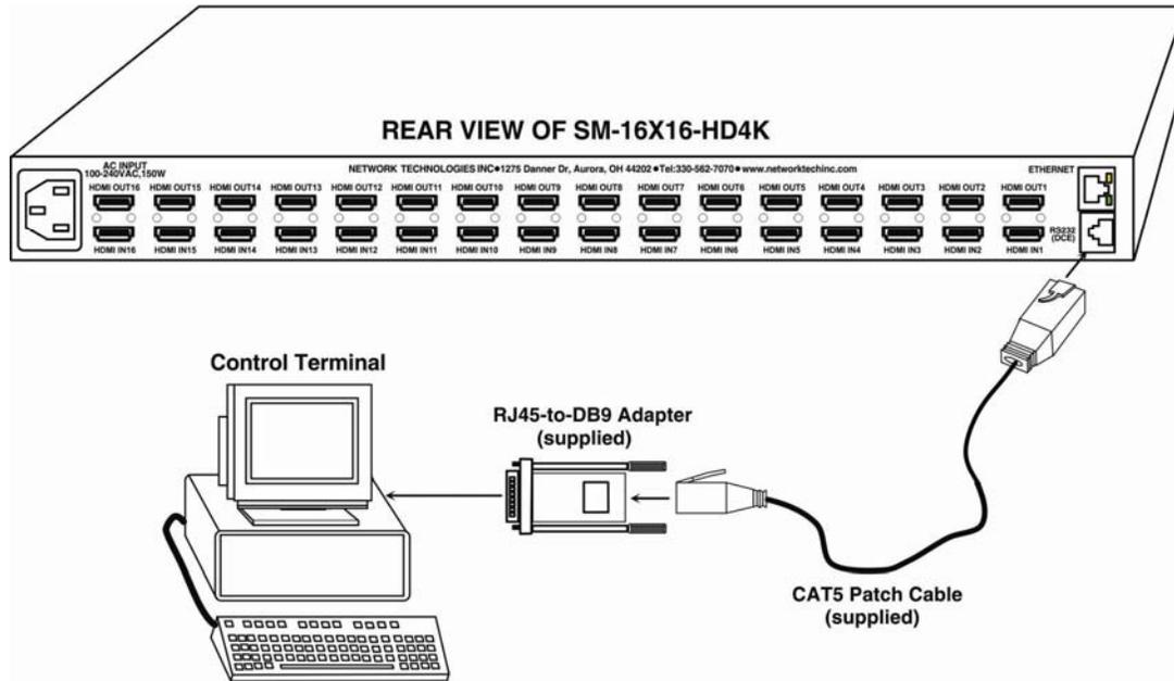
Figure 4- Connect RS232 control terminal to VEEMUX
