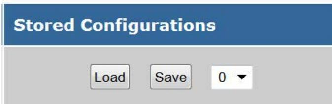
**Note:** This will save the currently active configuration on the VEEMUX and the DDC configuration (page 32). If changes have been made in the web interface without first pressing the **Submit** button, those changes will not yet be part of the active configuration.
