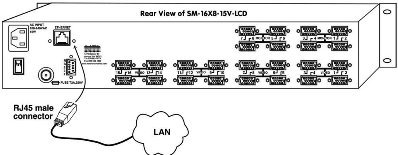
Figure 4- Connect the LAN to the VEEMUX
