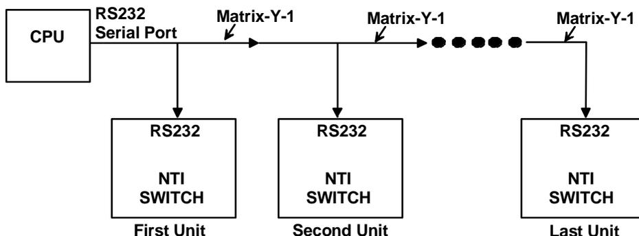
Figure 6- RS232 connection with Matrix-Y-1 cable
