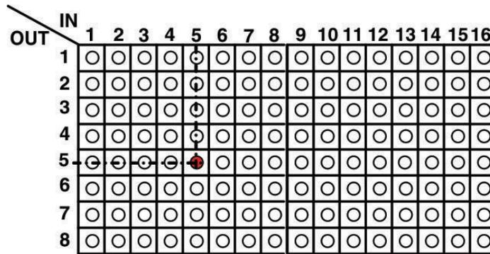
Figure 5- LED Matrix showing input 5 connected to output 5
