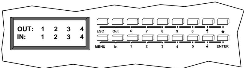
The following examples show various method of routing output 3 to input 5. Inputs and Outputs can be entered as a two digit number or a one digit number followed by IN or ENTER.
