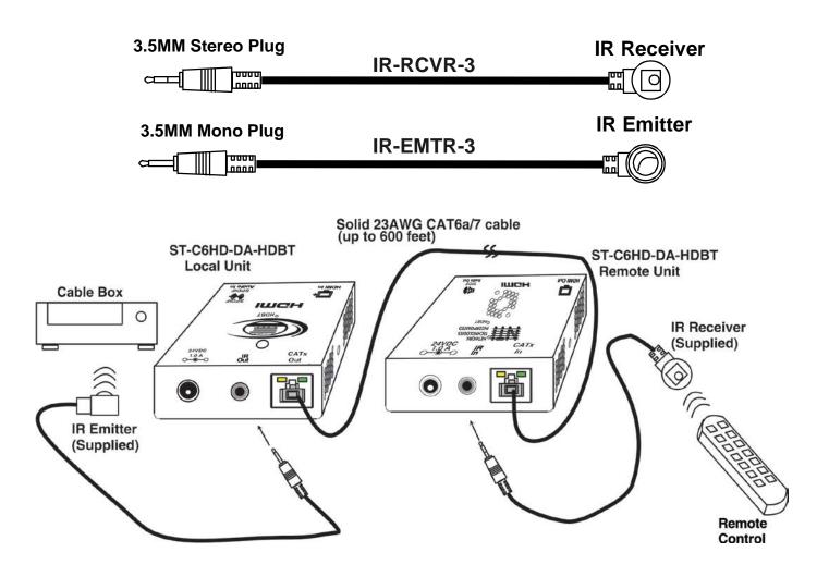
Figure 8- Connect IR Emitter and Receiver
