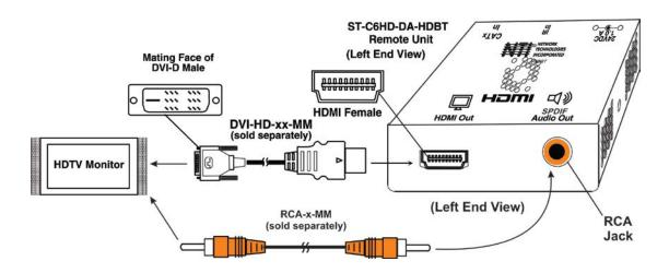
Figure 2- Installation with DVI-only monitor
