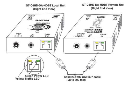
Figure 4- Connect CATx cable
