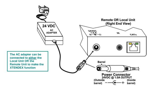
Figure 7- Connect the AC adapter to either the Remote Unit or the Local Unit
