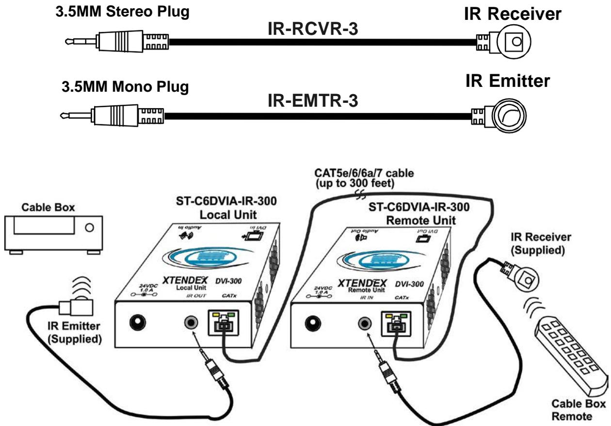
Figure 5- Connect IR Emitter and Receiver (models with IR support only)
