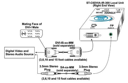
Figure 2- Connect the XTENDEX Local Unit to the source
