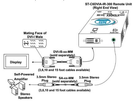
Figure 1- Connect the extended video display to the Remote Unit
