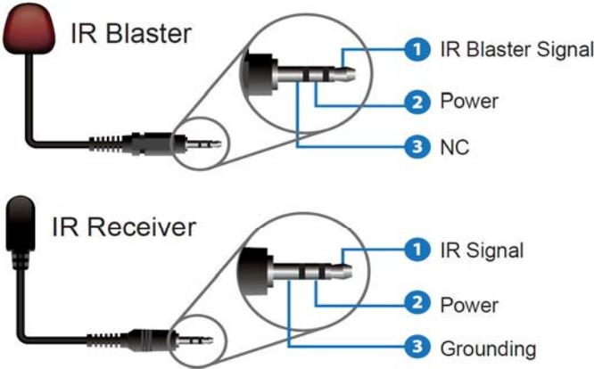
**Note:** When the angle between the IR receiver and the remote control is  $\pm 45^\circ$ , the transmission distance is 0-5 meters; when the angle between the IR receiver and the remote control is  $\pm 90^\circ$ , the transmission distance is 0-8 meters.
