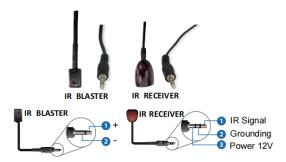
Note: When the angle between the IR receiver and the remote control is  $\pm$  45 °, the transmission distance is 0-5 meters; when the angle between the IR receiver and the remote control is  $\pm$  90 °, the transmission distance is 0-8 meters.
