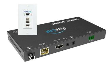
The HW-100 HDBaseT extender system provides 130 feet of 4K60 4:2:0 or 4K30 4:4:4 and USB 1.1 / 2.0. The HW-100 can also extend 1080P60 4:4:4 up to 230 feet. There are two USB-A ports on the transmitter that provide charging only functionality. The wall plate transmitter is powered by the receiver (PoC).
