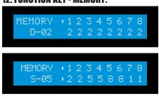
The system will show stored presets, up to a total of (16). Presets are stored in local memory using Source keys 1 thru 8 or Destination keys 1 thru 8 as the memory preset location.
