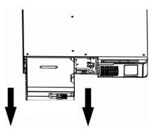
5. Slide in replacement battery pack. Refer to the figure directly below:
