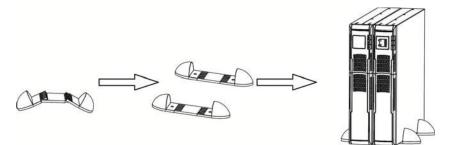
**NOTE:** When installing the UPS or external battery pack with feet, please keep both feet a distance of 2.75in (70mm) from the edge of the unit. See figure below:
