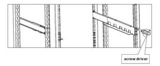
**Step 2.** Use four M6 screws to mount the right and left rail sliders to the two back posts of the four-post rack. Refer to the figure directly below:
