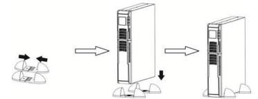
B.To install a UPS module and one extended battery pack, refer to the figure directly below : Assemble two feet each with an extension as one tower stand. Align the two stands.
