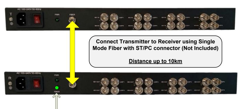
"FIBER" LED on the Receiver indicates that fiber is properly connected
