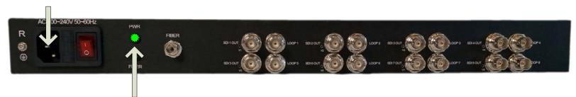
"PWR" LEDs on both units indicate that power is properly connected
