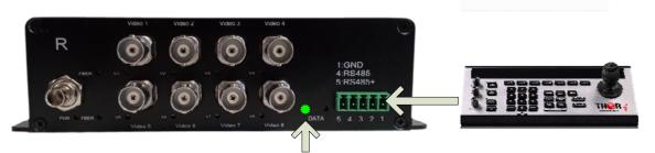
"DATA" LEDs on both T and R indicate RS data is properly connected
