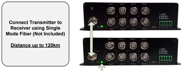
"FIBER" LEDs on both T and R indicate fiber is properly connected
