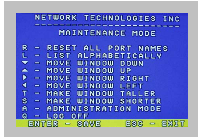
Figure 26- Maintenance Mode screen
