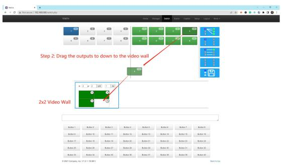
Users can have multiple video walls by the same way to create, for the 9x9 matrix switcher, the video wall configuration will be limited to 9, it means the configuration could be 3x4 video wall.
