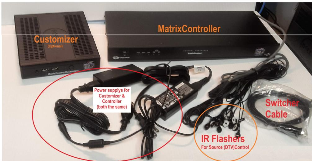
**Installation:** First connect the controller to a DHCP enabled network (most networks have this), then apply power. Next use the supplies DB9 Serial cable to connect your video matrix to port "A". Finally stick the prewired IR Flashers to the source receivers. The flashers are marked DTV1, DTV2, DTV3, etc. Be sure to put the DTV1 flasher on the DTV that is connected to input 1 on your matrix. DTV2 with flasher 2 must be hooked to input 2 and 3 to 3, and so forth.
