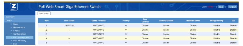
Configure the properties of the specified ports in batches (click the <Batch Configuration> button on the main page to enter the corresponding configuration page).
