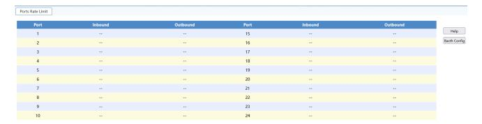
Configure the inbound/outbound port speed limit of a single port: click the entry corresponding to the port on the main page to enter the corresponding page.
