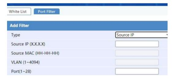
Before enabling the port filtering function, add the IP address and MAC address of the management device to the white list in the "White List Display Page" Device Information.
