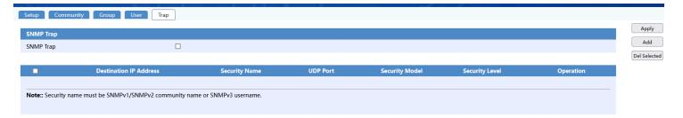
Click "New" to enter the new Trap host page, the user can configure the IP address, security name, UDP port, security model, the security level of the new Trap host.
